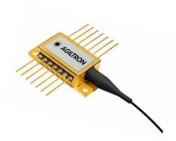
The 775nm series laser diodes are fabricated in a hermetically sealed 14-pin butterfly package. The laser diodes contain a monitor photodiode, thermoelectric cooler (TEC), and a thermistor to secure high-quality laser performance. Our laser products are Telcordia GR-468 qualified and in compliance with RoHS Directives.
